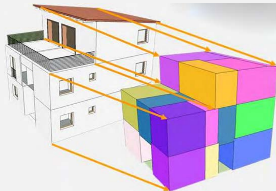
Fig. 27 3D view of an imported or newly drawn architectural model in the “3D Room Tool.” The tool recognizes rooms and building physics components with adjacent room relationships and adjusted dimensions, as required for SOLAR-COMPUTER calculations.
